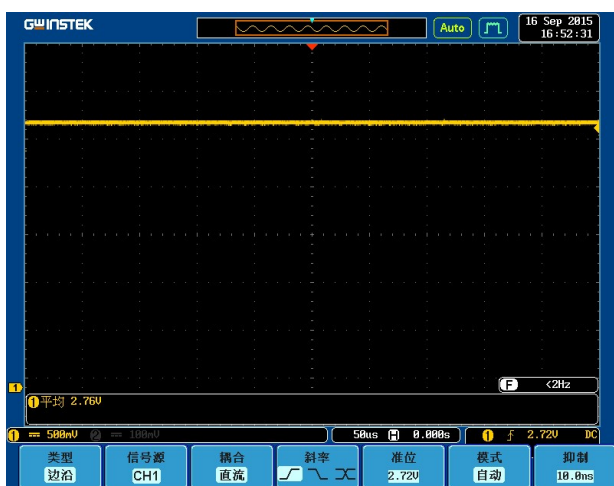
Fig. 16. The Closed-loop Output Current Waveform Of Buck Circuit
