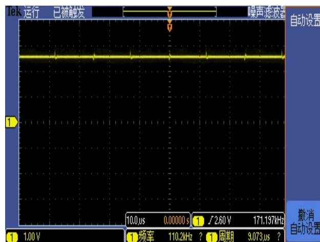
Fig. 14. The Open-loop Output Current Waveform Of BUCK Circuit
